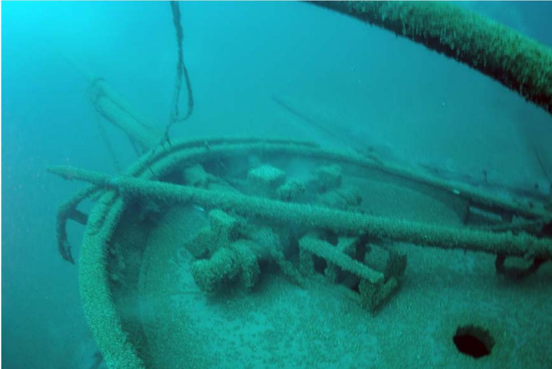
Figure 14. Windlass, bowsprit, and jibboom viewed from aft. The yard is visible lying across the windlass and the forecastle companionway.
